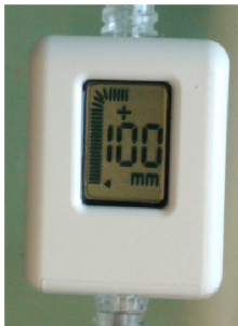
Figure 7: The “Compass™ Vascular Access” Device manufactured by Mirador Biomedical, Inc. This single-use device measures the intravascular pressure, which is displayed digitally and also as an analog representation of the pressure waveform. A guidewire may be passed through a separate valved port allowing continuous pressure measurement during the placement of the wire.
