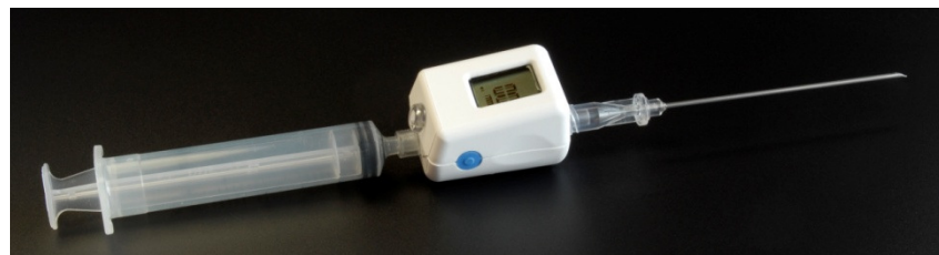
Figure 7: The “Compass™ Vascular Access” Device manufactured by Mirador Biomedical, Inc. This single-use device measures the intravascular pressure, which is displayed digitally and also as an analog representation of the pressure waveform. A guidewire may be passed through a separate valved port allowing continuous pressure measurement during the placement of the wire.
